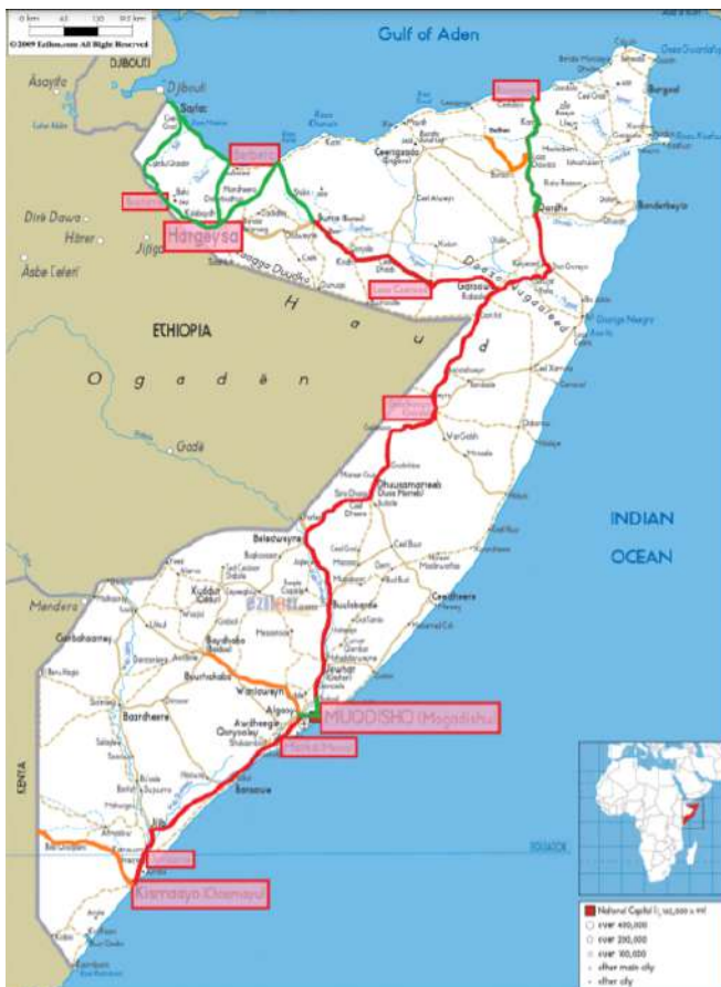
Figure 1 Fiber Optic Backbone Connecting 10 Cities
